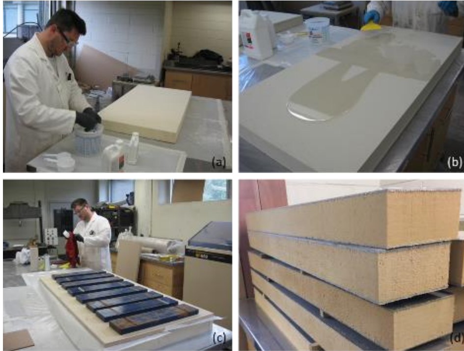
Figure 1. Specimen fabrication: (a) mixing epoxy and section of cleaned foam; (b) application of epoxy; (c) specimen curing with weighted board; and (d) finished specimens
